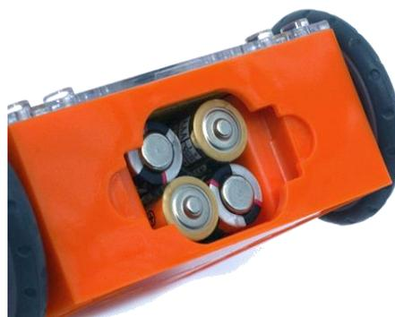
Ensure the batteries are in the right way.
